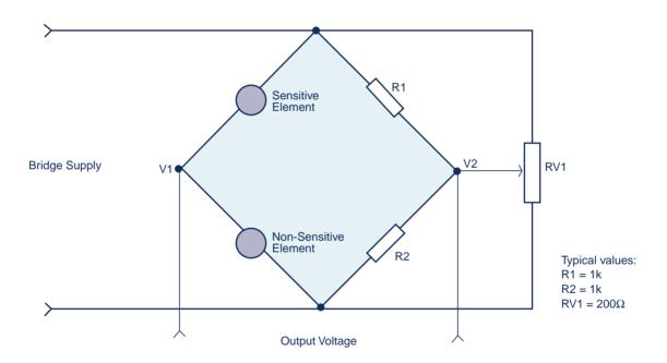
The Bridge Supply is typically 2.0 to 3.5 volts, depending on the sensor. Voltage V1 is set by the potential divider of the sensitive and non-sensitive elements and when no gas is present, this is nominally half the bridge supply voltage. Voltage V2 is also half the bridge supply and is predominantly determined by the potential divider of R1 and R2. RV1 is used to fine tune V1 and V2 so that they are the same value when no gas is present and enables the bridge output to be set to zero.
