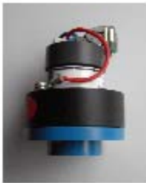
Fig 2. O 2 transmitter with blue installation ring
