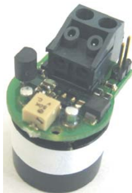
Fig 1. NO 2 sensor + 4-20 mA p.c.b. and screw terminals
