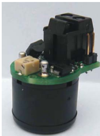
Fig. 1 ECO-Sure CO sensor + 4-20 mA p.c.b.
