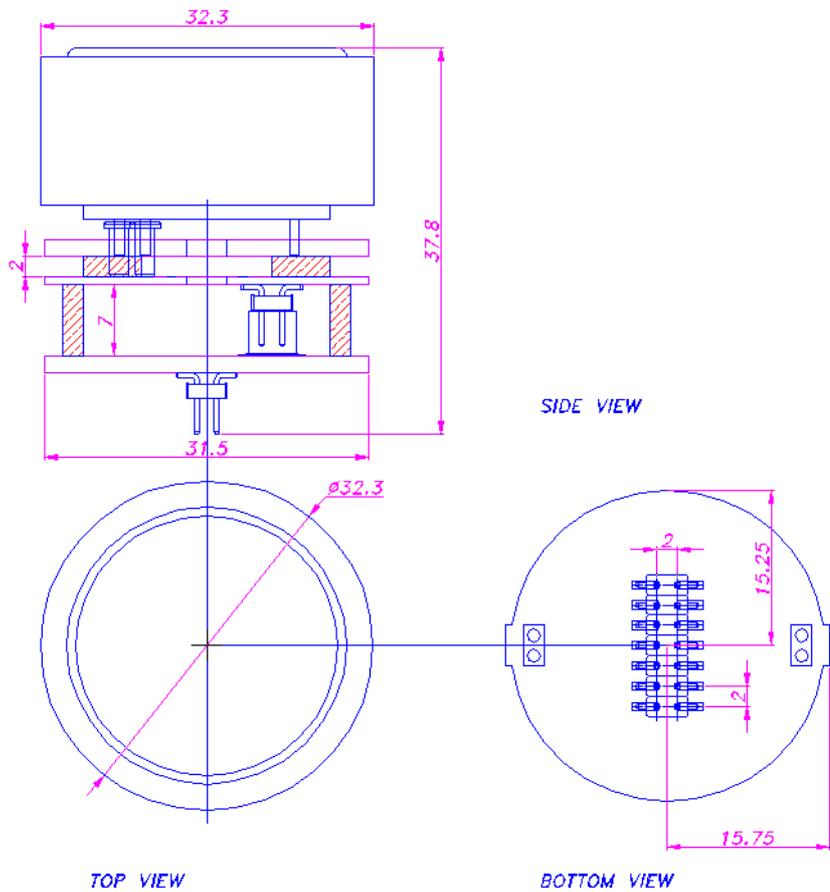
Figure 6.4 Electrochemical cell, 7 series type, for toxic gases detection;
