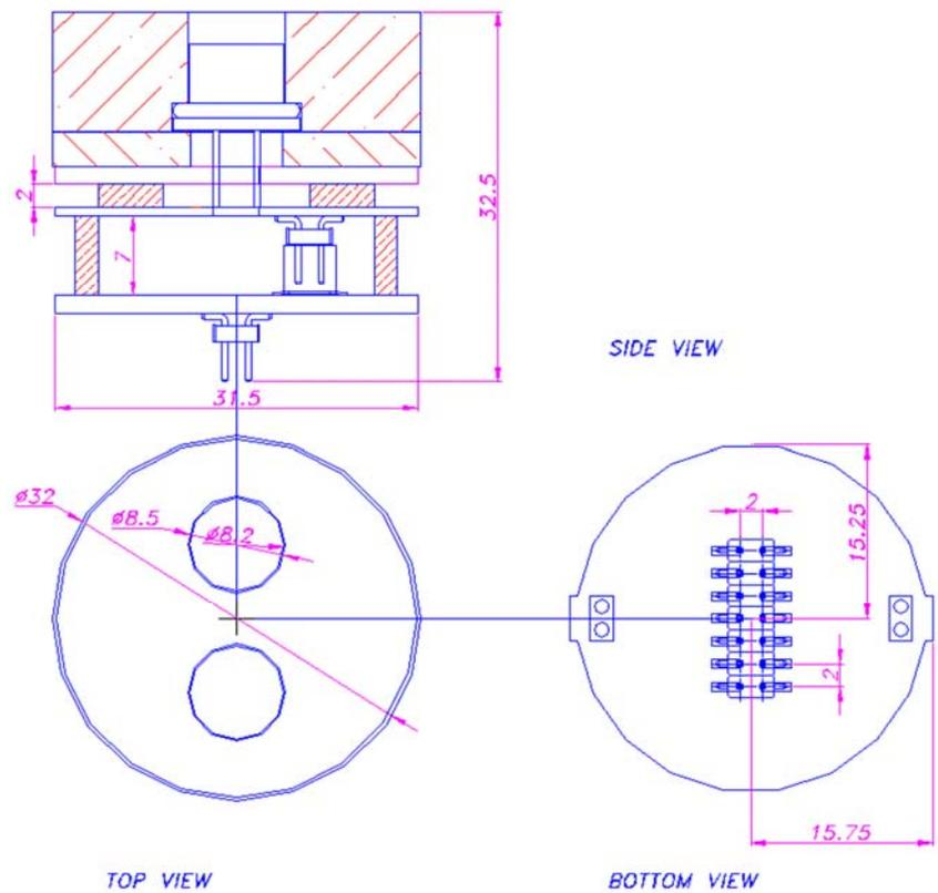
Figure 6.2 Twin industrial catalytic sensor for combustible gases;
