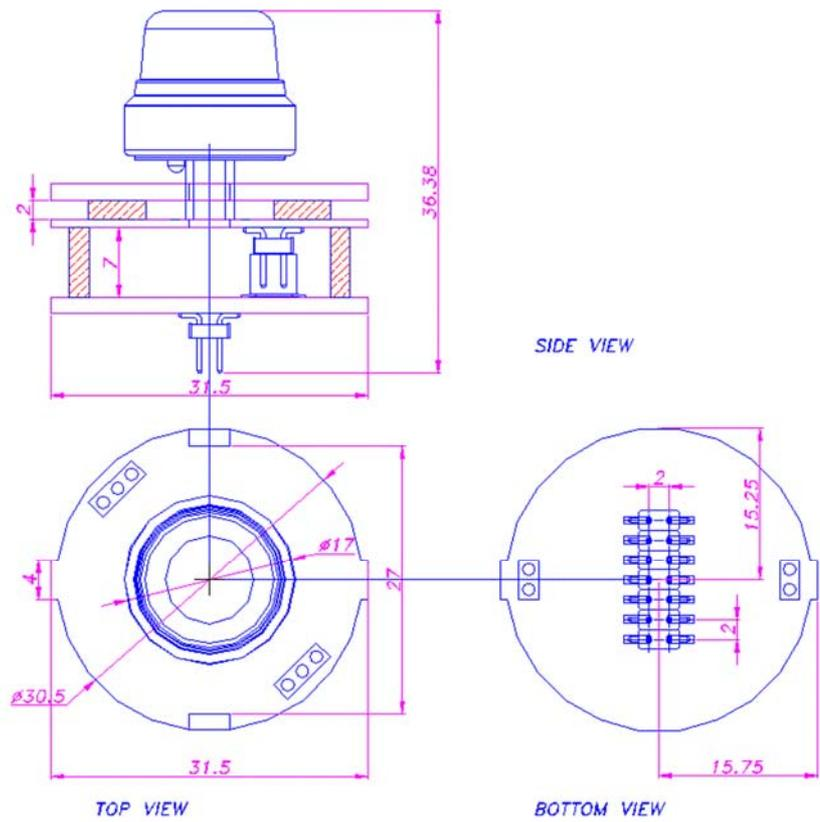
Figure 6.1 Single header industrial catalytic sensor for combustible gases;
