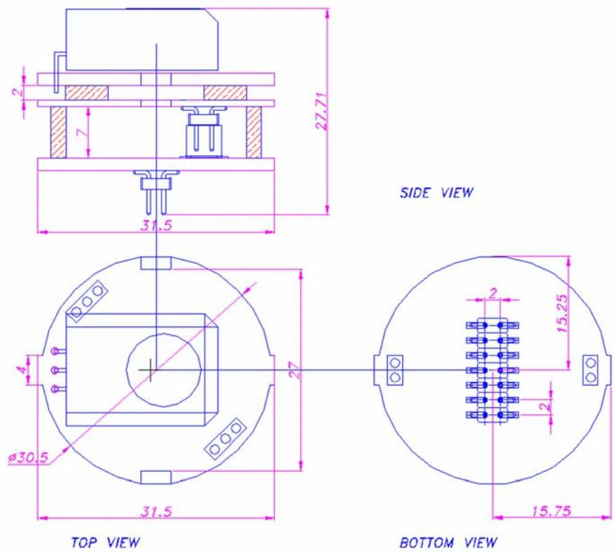
Figure 6.5 Electrochemical cell, flat series type, for toxic gases detection
