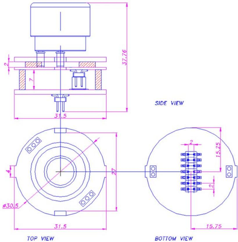
Figure 6.3 Electrochemical cell, 4 series type, for toxic gases detection;
