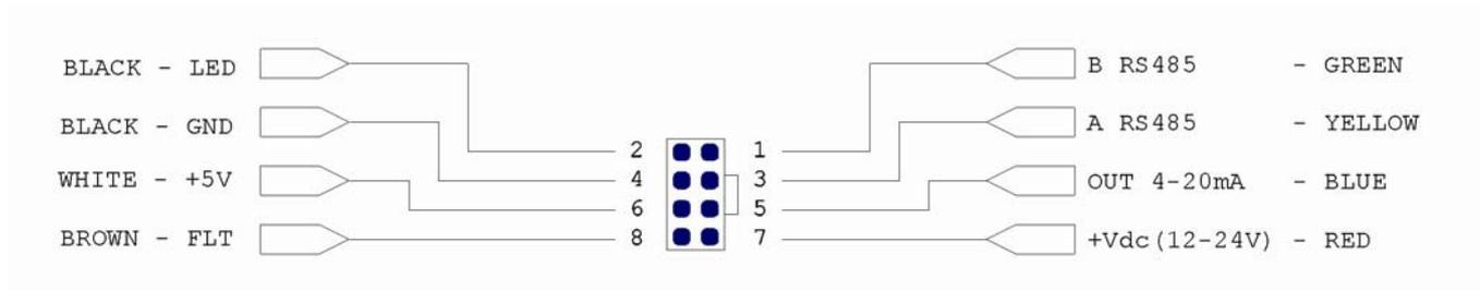
Figure 7.2. Cyber head cable connector.
