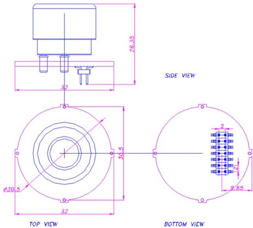
Figure 6.2 Electrochemical cell, 4 series type, for toxic gases detection;
