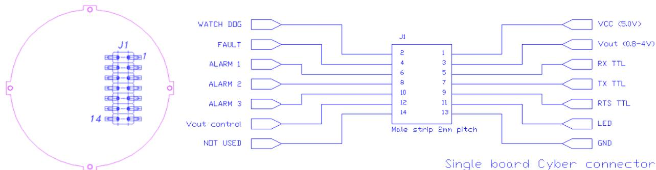
Figure 7.1 Single board Cyber connector and overview.
