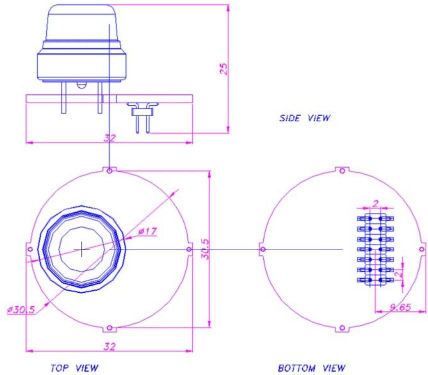
Figure 6.1 Single header industrial catalytic sensor for combustible gases;
