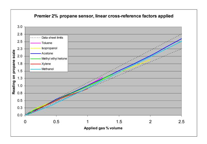
Note that in all the above examples, the temperature compensation is based upon propane, and there may be errors at temperatures away from the calibration temperature.
