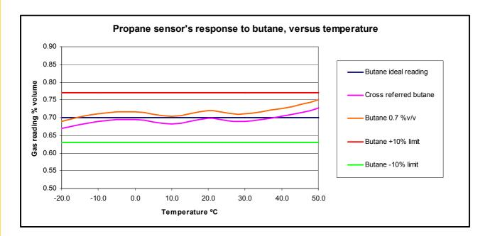
The above graph shows the output of a propane sensor, both with and without a cross-reference factor applied, against ambient temperature when tested with 0.7% volume butane.
