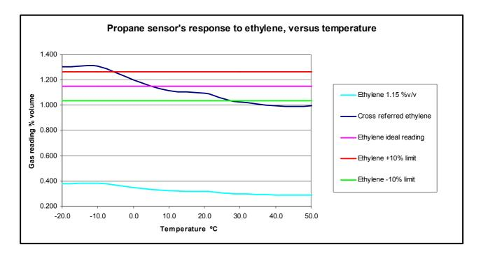
The above graph shows the output of a propane sensor, both with and without a cross-reference factor applied, against ambient temperature when tested with 1.15% volume ethylene.
