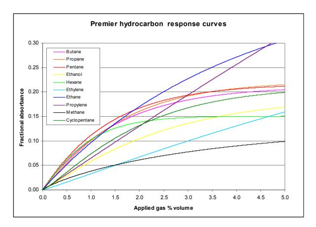
The above graph demonstrates the hydrocarbon sensor's fundamental response to a selection of gasses, before any linearisation is applied.
