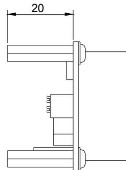
Figure 6. Side view of mounting to the base of an enclosure.
