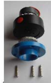
Fig 3. O 2 transmitter with sinter metal disc and blue installation ring
