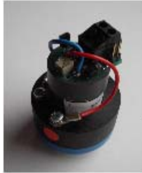
Fig 1. Oxygen transmitter with top ring for pcb and lower installation ring
