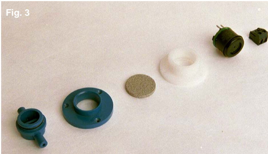
Fig. 3: Components from left to right: test gas cap; installation ring; sinter metal disc; sensor holder; ECO-Sure CO sensor with O-Ring and 4-20mA transmitter; pluggable terminal block.
