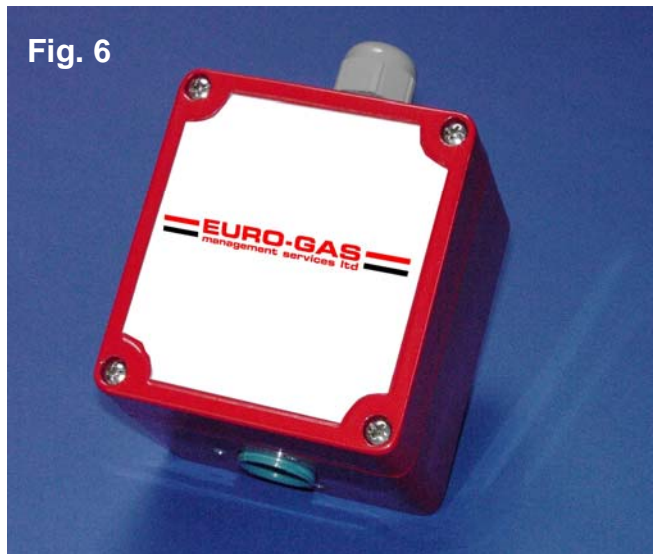
Fig. 6: ECO-Sure CO sensor with 4-20mA transmitter and installation kit, provided as a complete unit, fitted into Euro-Gas aluminium housing. Standard measuring range: 0-300ppm. Optional measuring range: 0-500ppm. Part no. 2112B1013
