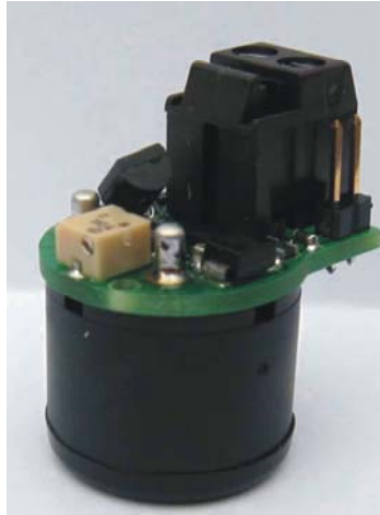
Fig. 1 ECO-Sure CO sensor + 4-20 mA p.c.b.
