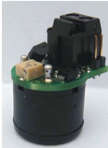
Fig. 1 ECO-Sure CO sensor + 4-20 mA p.c.b.
