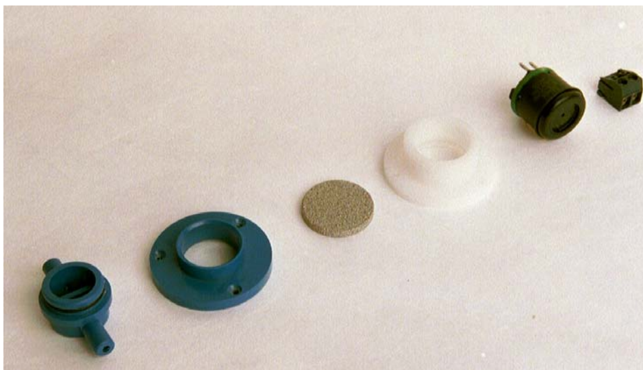
Fig. 3 Components from left to right: test gas cap, installation ring, sinter metal disc, sensor holder, ECO-Sure CO sensor with O-Ring + 4-20mA p.c.b. and plugable terminal block
