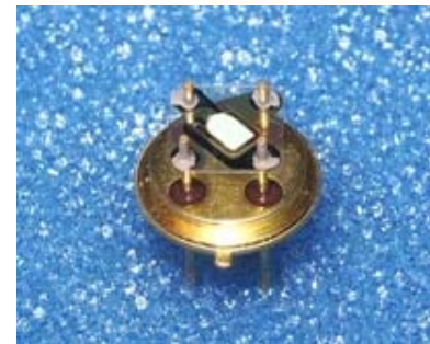
Figure 1: Agricultural ammonia sensor packaged on a TO-39 header.
